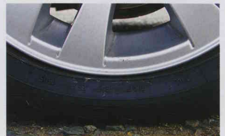
Goodyear's RunOnFlat works using a reinforced sidewall so that the tyre retains some shape, even when flat
